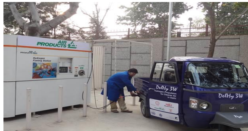
Hydrogen Filling station by Indian oil and Hydrogen fuelled three wheeler by IIT Delhi and Mahindra & Mahindra
